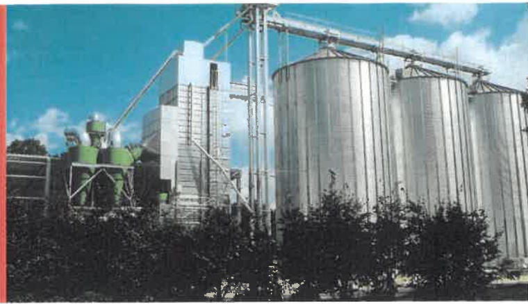
Romberger® drying system with Romberger® conveyor technology and silos Pöhlking Manor, Steinfeld Ortenburg
