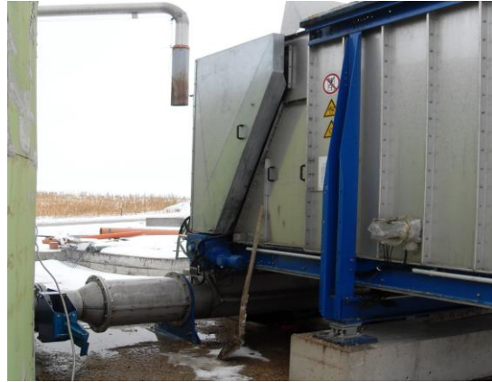
Solid material metering feeder with screw press
