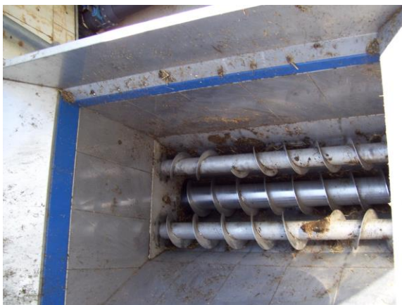
Feeding hopper with feeding rollers
