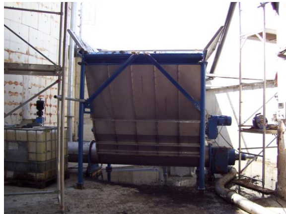
Feeding hopper 10 m 3 with screw press
