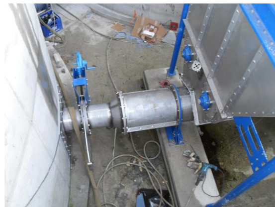
Feeding hopper 10 m 3 with screw press
